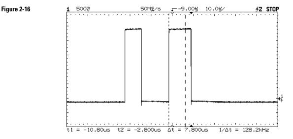
By moving the time cursors together, you can check for pulse width variations in a pulse train, as figures 2-15 and 2-16 show.
