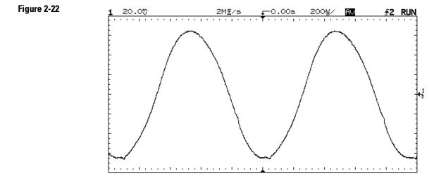
On this waveform, 256 averages were used to reduce the noise
