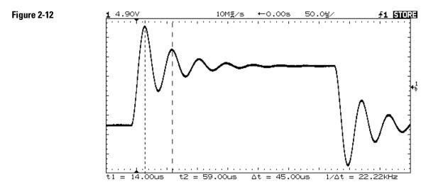
Cursors used to measure the frequency of the ringing on a pulse
