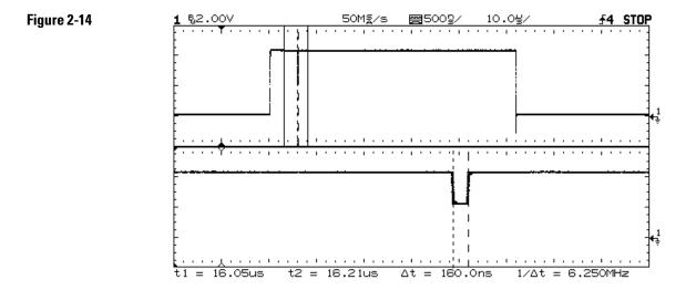
The cursors track delayed sweep. Expand the display with delayed sweep, then characterize the event of interest with the cursors.
