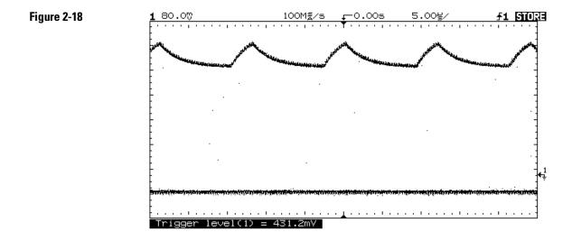
This is a triggered view of the asynchronous noise shown in figure 2-17.
