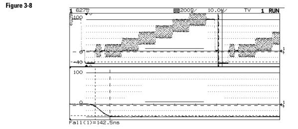
Modulated staircase or 5-step, measuring sync pulse fall time with delayed sweep
