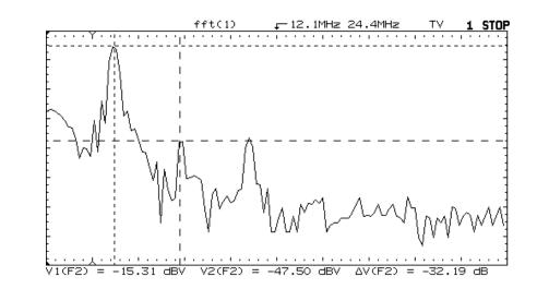
The FFT function shows that the harmonic content of the color busrt is more than 31 dB below the subcarrier
