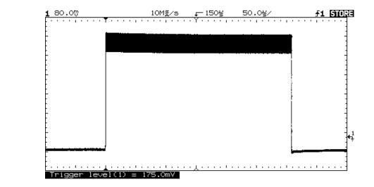
Asynchronous noise at the top of the pulse
