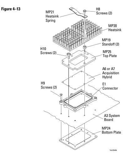
A6/A7 Acquisition Hybrid and associated mounting parts
