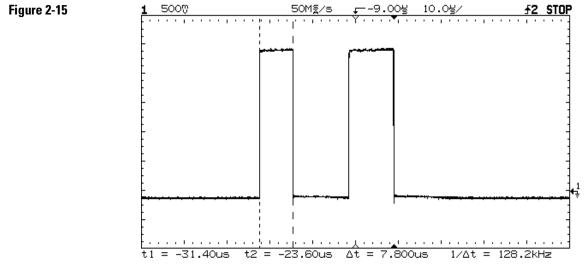
Pressing t1 and t2 softkeys simultaneously causes the time cursors to move together when the cursor knob is adjusted.
