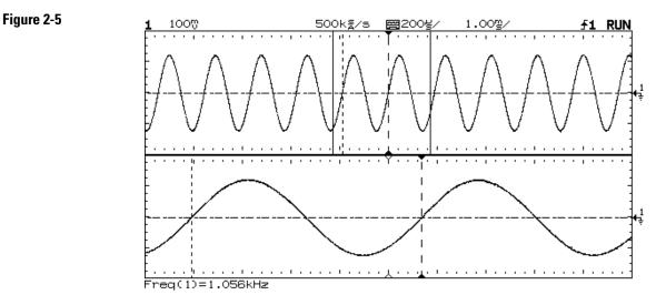
Delayed time base isolates an event for a frequency measurement
