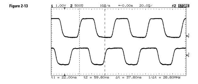
Cursors used to make channel-to-channel delay measurements
