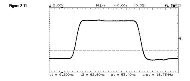
Cursors used to measure pulse width at levels other then the 50% points
