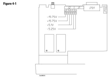
Low Voltage Power Supply voltage test points (bottom side of oscilloscope)
