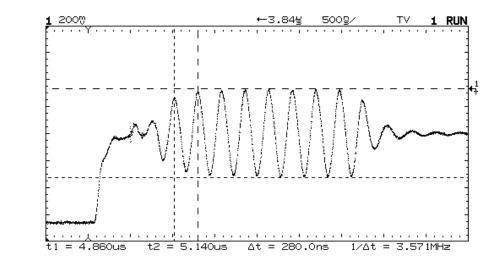
The scope controls are used to zoom in on the color burst in the time domain
