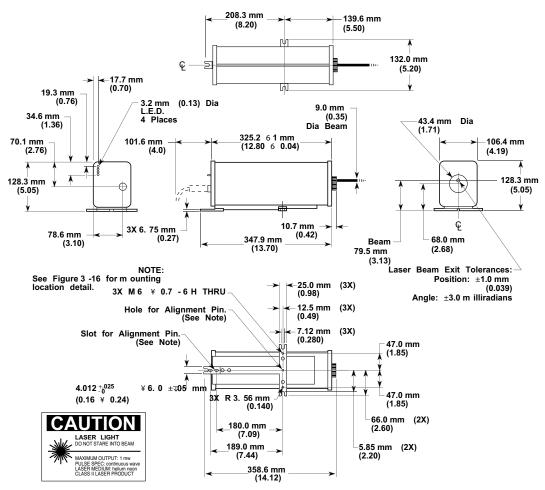
Figure 5-7B. Agilent 5517C-009 Laser Head dimensions
