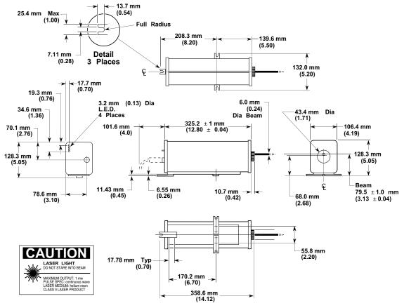
Figure 5-7A. Agilent 5517C Laser Head, (Standard and 5517C-003) dimensions
