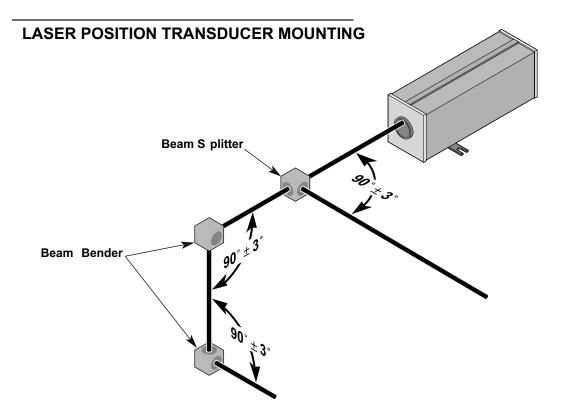
Figure 5-1. Laser position Transducer mounting
