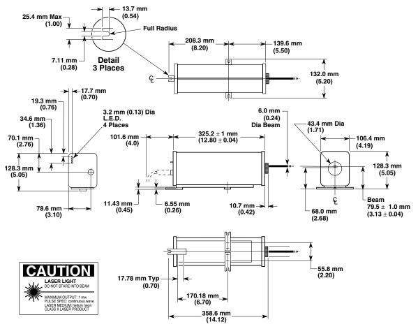
Figure 5-5. Agilent 5517B Laser Head dimensions
