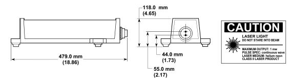
Figure 5-12. Agilent 5519A/B Laser Head dimensions
