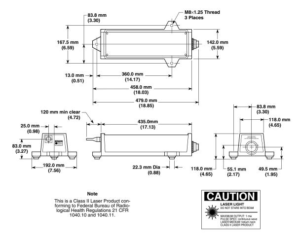
Figure 5-3. Agilent 5517A Laser Head dimensions
